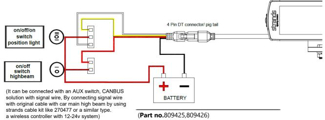
\*No fuse, 15cm cable with DT4 and pig tail, No hello function
