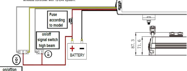
(**Part No.**809427,809431 (25A fuse) 809428,809429,809432,809433 (40A fuse) 8094030,809434 (50A fuse) , 2.5m cable, Hello function
