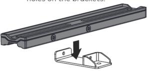
Where possible, always use the centre holes for attaching to Pivot Bracket. If extra clearance is needed due to Platform-to-roof fitment needs, the offset holes can be used.
