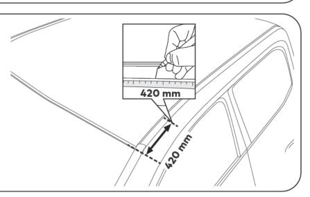
POSITION RUGGEDLINE ON ROOF CHANNEL
